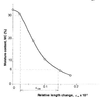
FIG. 1 Determination of Drying Shrinkage,  $\epsilon_{\rm cs}$
